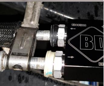
Inspect original O-ring on the tube, replace with supplied viton O-ring (1453153) if it is damaged.
